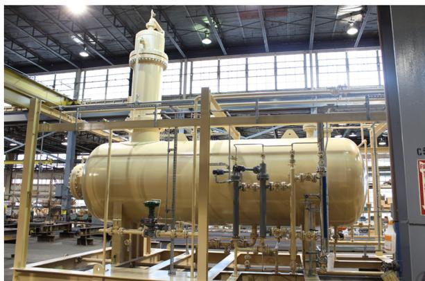
**Figure 1.** A typical single-stage FIBER FILM Contactor – the vertical pipe mounted on top of the horizontal phase separator. Untreated hydrocarbon and fresh treating solution enter at the top. Treated hydrocarbon and spent treating solution exit from the top and bottom of the separator, respectively.
